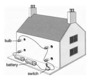
(a) When Alice turns the switch on, the bulbs do **not** light up. The batteries are **not** flat. None of the bulbs is broken. Why do the bulbs **not** light up?
